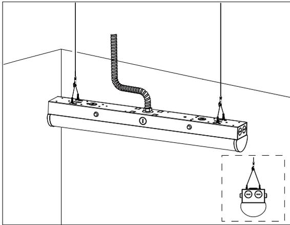
1. Fixing the hook and suspending the lamp.
