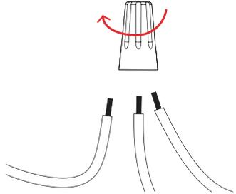
11. Tighten the wires in the wire nut as the photo shows below.
