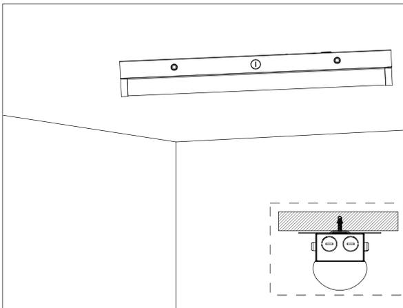
1.Punch a hole on the wall and put the expansion tube inside.For reference, mounting holes are spaced 36 1/4" on 4FT model and 83 3/8" apart on the 8FT model.
