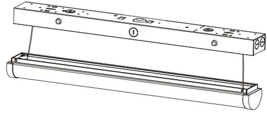
3.Run the fixture's power wires through the center hole. of the round J-box adapter. Slide and secure the round J-Box adapter on the center slots located on the back of the fixture.
