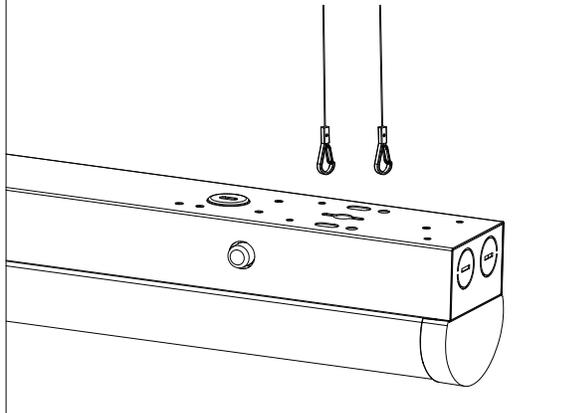
4. Turn off the power and make wiring by using wire nuts according to wiring diagram
