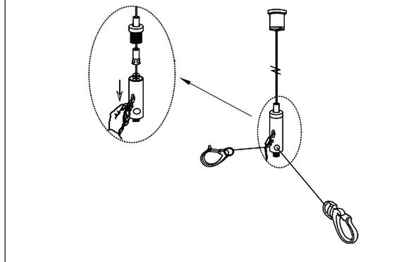
3. Adjusting the safety rope making the LED Strip in a horizontal state.
