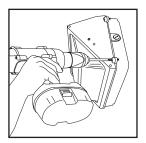
**STEP 6** Tighten two captive screws on side of housing.
