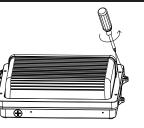
2.Use a screwdriver to remove the screws on both sides and remove the upper cover of the fixture.
