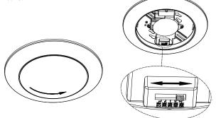
3. Recessed Can Installation: Attach the friction clips(not included) to the fixture. Adjust arrow on the clips to align with the number on the fixture in order to achieve a tight fit inside the housing. (5" and 6" refers to the 5" and 6" can housing installation hole)
