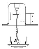
8. Carefully place wires into fixture and push the fixture into the housing until flush with ceiling.
