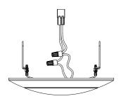
6. Screw E26 base adapter (not included) into socket in recessed housing, and simply slide the trim and torsion springs into the housing.
