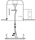
7. Carefully place wires into fixture and push the fixture into the housing until flush with ceiling.
