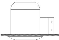
8. Caulk around the mounting surface edge with silicone sealant.
