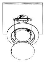
6. Replace lens and twist counter clockwise to lock. Caulk around the mounting surface edge with silicone sealant.
