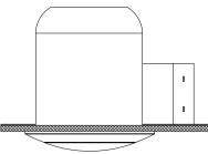
8. Caulk around the mounting surface edge with silicone sealant.
