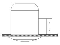
9. Caulk around the mounting surface edge with silicone sealant.
