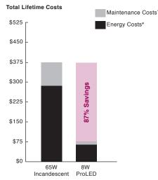
Y Maintenance costs based on 15 minutes at \$40 per/hr ¥ Energy costs based on \$0.11 kWh
