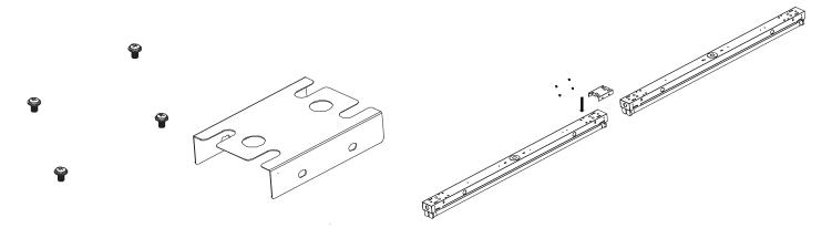
3. Attach the bracket to the fixtures using (4) supplied screws.
