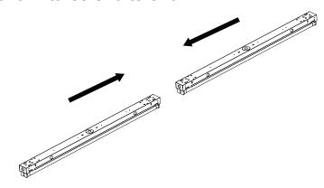
2. Slip mounting bracket over the ends of the fixtures, aligning screw holes on the side of the bracket with fixtures.
