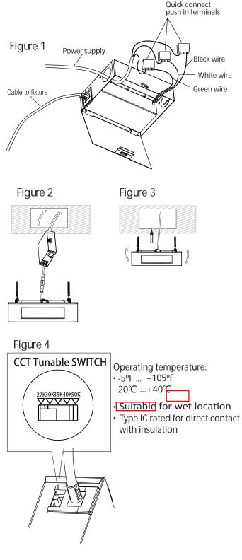
**WARNING:** For wet location installation, after fixture is installed on ceiling, put silicone glue to seal the gap between fixture and ceiling.
