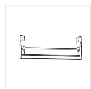
9.Insert the LED panel to the end. Fix the last frame and close the kit.
