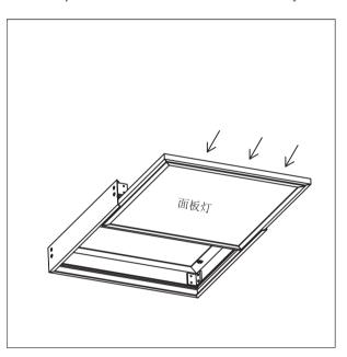
Please ensure the Length of driver connect line is long enough to avoid the unnecessary presure when slide the Panel light into frame.
