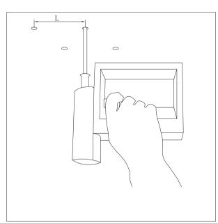
Please ensure the ceiling is concrete solid construction with thickness at least 50mm! Or it may cause the screw anchors loose, even fall out. The dia of hole can't ne larger than!
