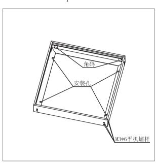
Please mind to assemble two frames with mounting holes in corresponding two sides to avoid slipping
