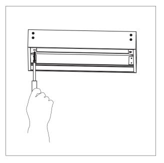
Note: the end cap must be well fixed by spanner, or, they may fall out with time going on.
