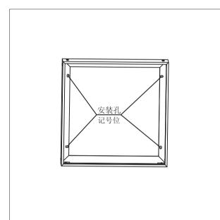
5.Put the screw anchors into corresponding holes and knock them into the ceiling by a hammer until the outer edge of the screws along ceiling surface
